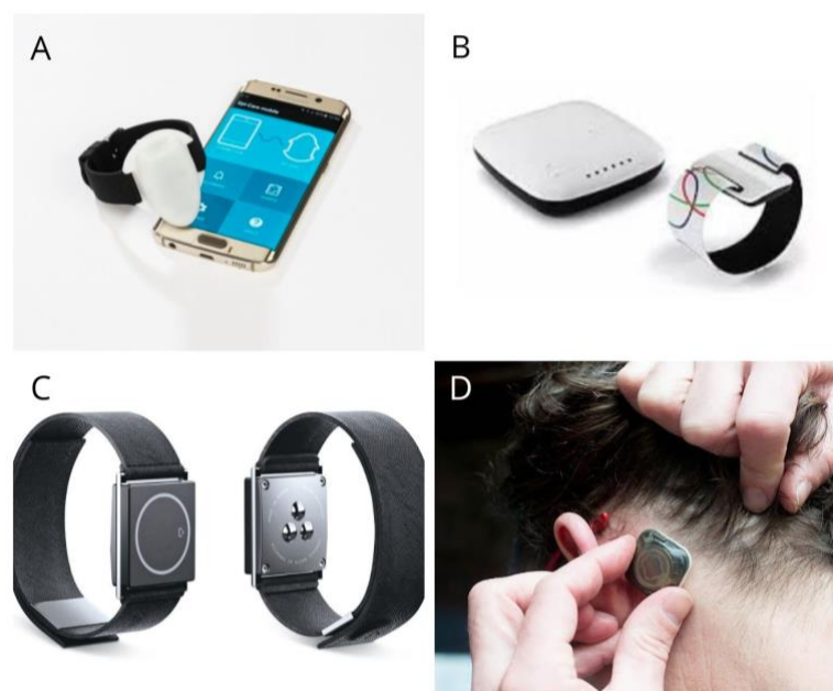
Fig. 1. A) Epi-Care mobile, sensing device based on 3D-acc B) NightWatch device based on both photoplethysmography (PPG) to measure heart rate and accelerometry data (ACC) C) Embrace Wristband, this device uses three-axis ACM sensor, a three-axis gyroscope sensor, and an EDA sensor D) EpitelEpilog - a wearable, wireless behind the ear, electroencephalography (EEG) sensor system
